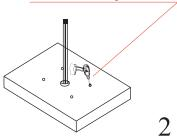
Drive the expansion screw into the cement pier.
