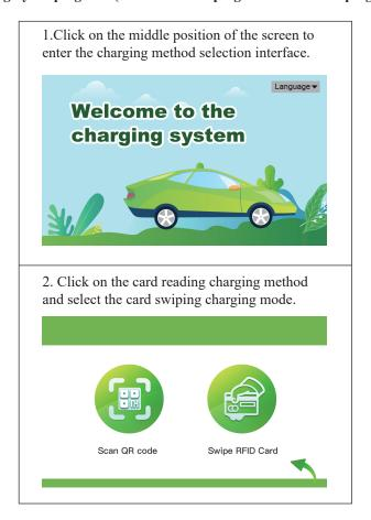
3. Enter the waiting card swiping to start charging interface. Waiting To Swipe The Card 4. Swipe card successfully and enter the charging interface. Charging Amount: Voltage: V/ac Current: Electric Quantity: kW∙h Charging Duration: Min 5. Swipe the card again to stop charging and enter the settlement interface. Card No.: Account Balance: \$ Order Amount: Charging Capacity: kW∙h Charging Duration: Min Prompt:
